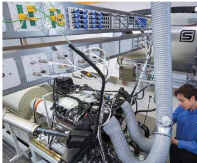
An engine being instrumented inside one of the newly installed engine test cells at Intertek, Milton Keynes, UK
