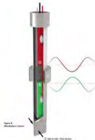
Figure B: Out Of Phase Vibration Signals
