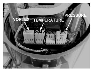
Figure 5-1. Electronics Stack Sensor Connections
