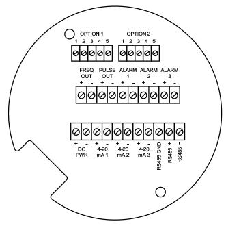
Figure 2-24. DC Wiring Terminals
