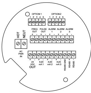
Figure 2-22. AC Wiring Terminals
