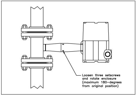
Figure 2-13. Enclosure Viewing Adjustment
