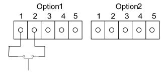
Figure 2-41. Optional Contact Closure Input Wiring
