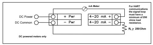
Figure 2-28. Non-Isolated 4-20 mA Output Using Meter Input Power Supply
