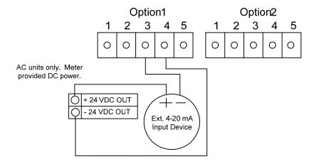
Figure 2-40. External 4-20 mA Input Wiring - AC Powered Meter
