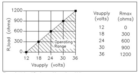
Figure 2-16. Load Resistance Versus Input Voltage
