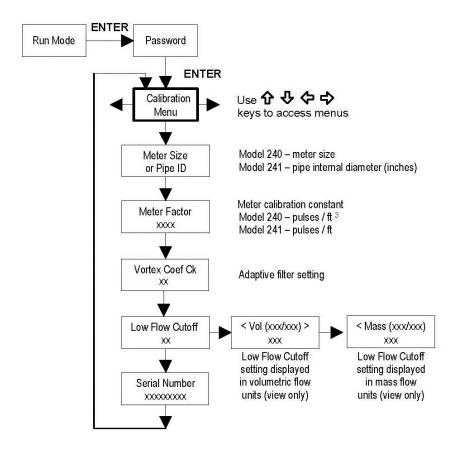
The Calibration Menu contains the calibration coefficients for the flow meter. These values should by changed only by properly trained personnel. The Vortex Coef Ck and Low Flow Cutoff are set at the factory. Consult the factory for help with these settings if the meter is showing erratic flow rate.
