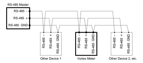
Figure 4-4.RS-485 Wiring (MODBUS)
