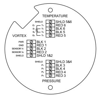
Figure 2-36. High Power Flow Meter Junction Box Sensor Connections
