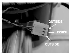
Figure 5-3. Vortex Sensor Connector
