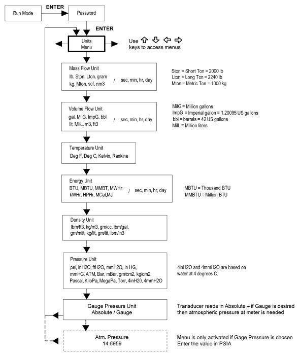
Use the Units Menu to configure the flow meter with the desired units of measurement. (These are global settings and determine what appears on all screens.
