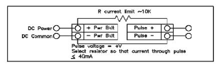
Figure 2-18. Non-Isolated Pulse Output Using External Power Supply
