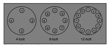
Figure 2-2. Flange Bolt Torquing Sequence
