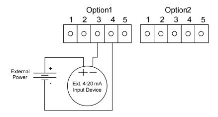
Figure 2-38. External 4-20 mA Input Wiring - External Power Supply
