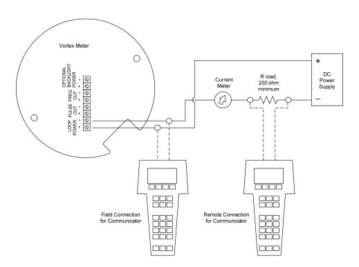
Figure 4-1.Loop Powered Meter Wiring (HART)
