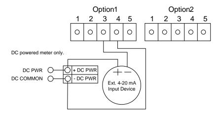
Figure 2-39. External 4-20 mA Input Wiring - DC Powered Meter
