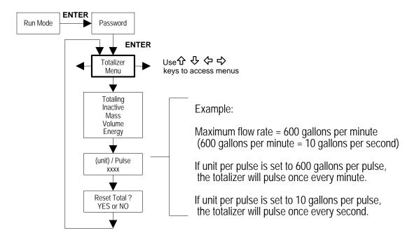
Use the Totalizer Menu to configure and monitor the totalizer. The totalizer output is a 50 millisecond (.05 second) positive pulse (relay closed for 50 milliseconds). The totalizer cannot operate faster than one pulse every 100 millisecond (.1 second). A good rule to follow is to set the unit per pulse value equal to the maximum flow in the same units per second. This will limit the pulse to no faster than one pulse every second.
