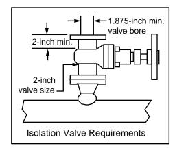
3. Choose an isolation valve with at least two inches existing between the flange face and the gate portion of the valve. This ensures that the flow meter's sensor head will not interfere with the operation of the isolation valve.
