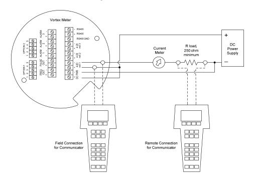
Figure 4-2.DC Powered Meter Wiring (HART)
