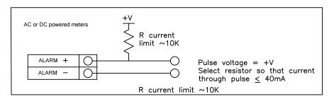
Figure 2-33. Isolated Alarm Output with External Power Supply
