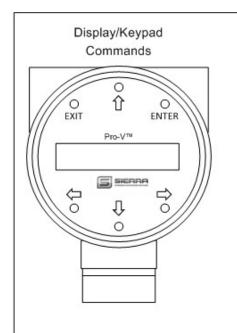
From the Run Mode, the ENTER key allows access to the Setup Menus (through a password screen). Within the Setup Menus, pressing ENTER activates the current field. To set new parameters, press the ENTER key until an underline cursor appears. Use the ① ① ⇔ keys to select new parameters. Press ENTER to continue. (If change is not allowed, ENTER has no effect.) All outputs are disabled when using the Setup Menus.
