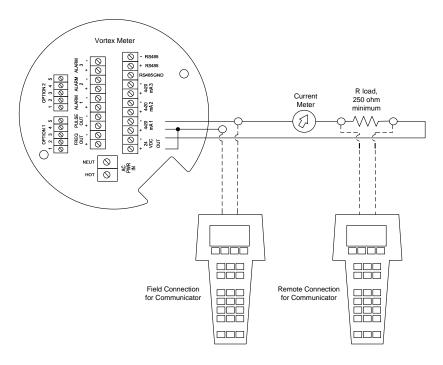
Figure 4-3.AC Powered Meter Wiring (HART)
