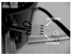
Figure 5-4. Temperature Sensor Connector
