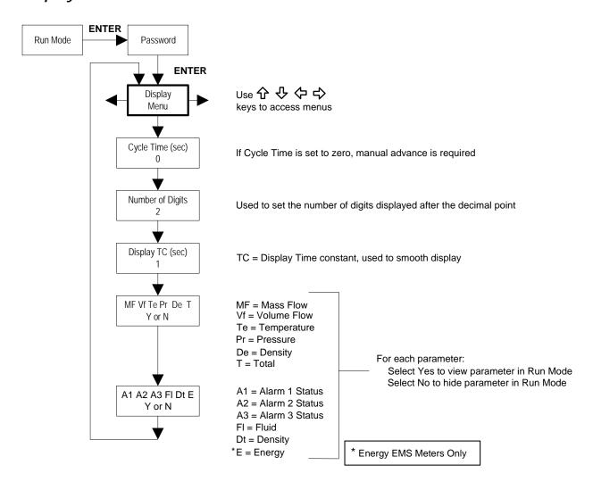
Use the Display Menu to set the cycle time for automatic screen sequencing used in the Run Mode, change the precision of displayed values, smooth the values or enable or disable each item displayed in the Run Mode screens.
