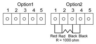
Figure 2-37. Optional Energy EMS RTD Input Wiring
