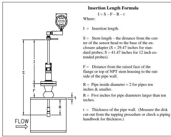
Figure 2-11. Insertion Calculation (Meters without Insertion Tool)
