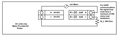
Figure 2-29. Isolated 4-20 mA Output using Meter Provided Power Supply
