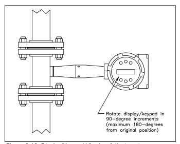
Figure 2-12. Display/Keypad Viewing Adjustment
