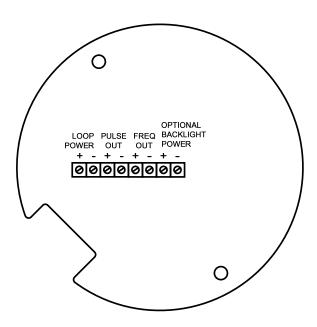
Figure 2-14. Loop Power Wiring Terminals
