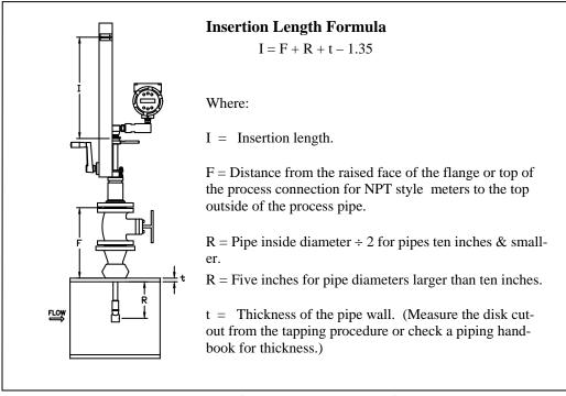
Figure 2-8. Insertion Calculation (Meters with Insertion Tool)
