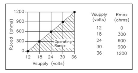
Figure 2-26. Load Resistance Versus Input Voltage
