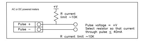
Figure 2-30. Isolated Pulse Output with External Power Supply
