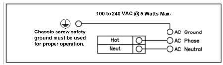
Figure 2-23. AC Power Connections
