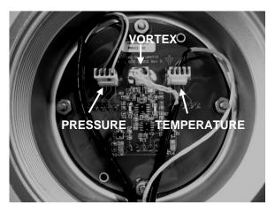
Figure 5-2.Remote Feed Through Board Sensor Connections
