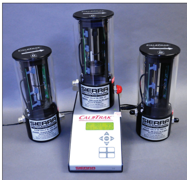
CalTrak Base with Three Flow Cells
