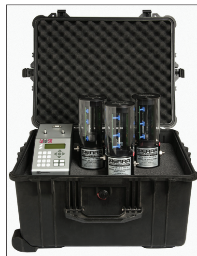
CalTrak Base with Three Flow Cells
