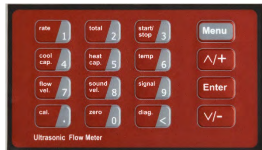
Figure 3. 16 Tactile Keys With 12 Dual-Function Keys
