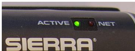
LED's showing the activities of the Compod™
