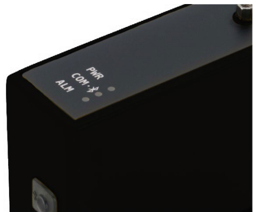
Figure 23 Top of unit where LED's are located
